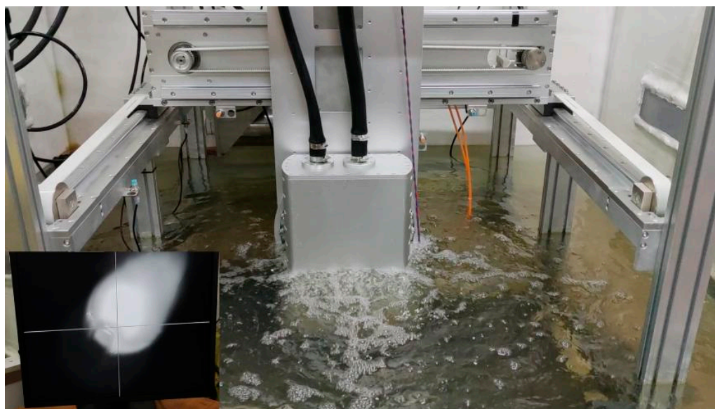
Figure 2. Underwater laser cladding system for underwater laser cladding/remelting processing.
