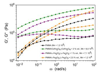
**Figure 9.** Variation of the storage  $G'(\blacksquare)$  and loss  $G''(\bullet)$  moduli of pure PMMA and of PMMA chains grafted onto the surface of NPs (PMMA/NPs), as a function of frequency  $\omega$  at a temperature of 210 °C.
