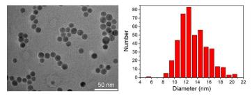
**Figure 4.** TEM image of iron oxide NPs (**left**) and size distribution measured on 436 NPs (**right**). The average diameter is 13.3 nm, and the standard deviation is 5.9 nm.
