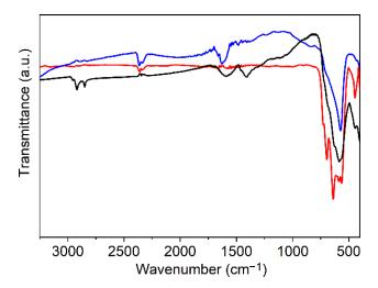
**Figure A7.** FTIR spectra with entire wavenumber range of iron oxide NPs (black) compared to spectra of neat magnetite (blue) and maghemite (red) powders. An expansion of spectra to wavenumber region of interest (900 to  $400 \text{ cm}^{-1}$ ) is shown in Figure 3.
