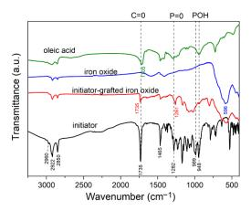
**Figure 5.** FTIR spectrum of initiator-modified iron oxide (red), compared to spectra of oleic acid (green), iron oxide (blue), and initiator (black).
