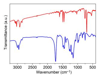
**Figure A6.** FTIR spectra of PS/ $\gamma$ -Fe<sub>2</sub>O<sub>3</sub> (red) and PMMA/ $\gamma$ -Fe<sub>2</sub>O<sub>3</sub> (blue) displaying the characteristic bands of the polymers.
