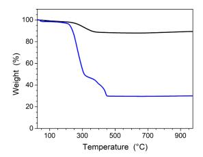
Figure A2. TGA curves of before (blue) and after (black) washing and size selection.
