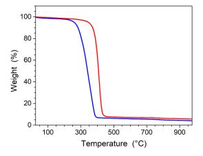
Figure A5. TGA of PS/ $\gamma$ -Fe<sub>2</sub>O<sub>3</sub> (red) and PMMA/ $\gamma$ -Fe<sub>2</sub>O<sub>3</sub> (blue). For a better accuracy, TGA experiments were combined to calcination of 20–25 mg sample amounts at 500 °C for one or several hours. Residual weight was constant after 1 h, giving an accurate iron oxide weight fraction confirming TGA results: 10.8 wt % (PS/ $\gamma$ -Fe<sub>2</sub>O<sub>3</sub>) and 9.5 wt % (PMMA/ $\gamma$ -Fe<sub>2</sub>O<sub>3</sub>).
