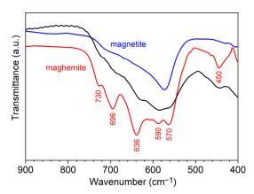
**Figure 3.** FTIR spectra of iron oxide NPs (black) compared to spectra of neat magnetite (blue) and maghemite (red) powders. Spectra with entire wavenumber range are displayed in Figure A7.
