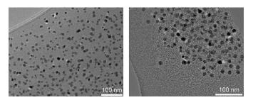
**Figure 6.** TEM images of PS/ $\gamma$ -Fe<sub>2</sub>O<sub>3</sub> (**left**) and PMMA/ $\gamma$ -Fe<sub>2</sub>O<sub>3</sub> (**right**).
