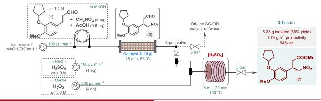
Scheme 5. Synthesis of (S)-Rolipram via Continuous Flow Metal-Free Nitro Reduction/Lactamization of 7
