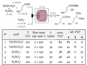
$^aH_2O_2\,$  added as 35 wt% aq solution.  $^bDetermined\,$  by HPLC area%.  $^cAdded$  as 6.0 M aq  $H_2SO_4\,$  solution.  $^dAdded$  as cc  $H_2SO_4.$
