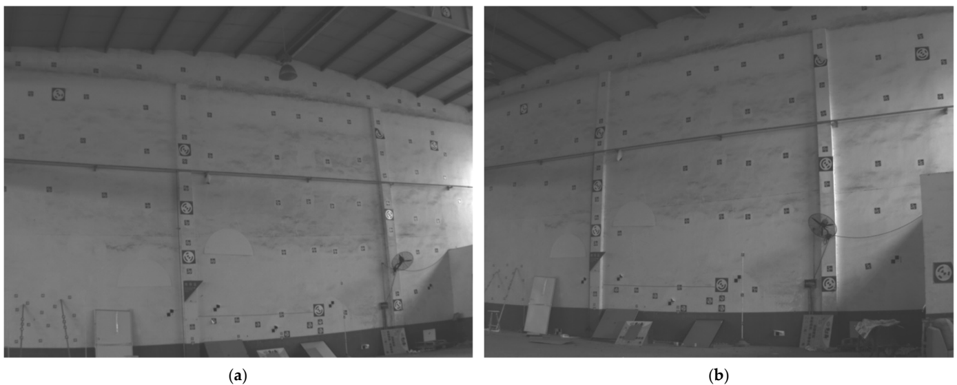
Figure 9. Real images with heavy distortion. (a) The real image captured by the first camera. (b) The real image captured by the second camera. Some control points are placed near the edges of both images.
