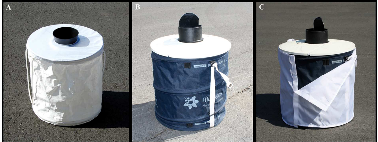
Fig 1. The three variations of the Biogents Sentinel trap. (A) Original BGS1. (B) PVC-coated BGS2P prototype (BGS2P). (C) PVC-coated BGS2P with optional white cover.
