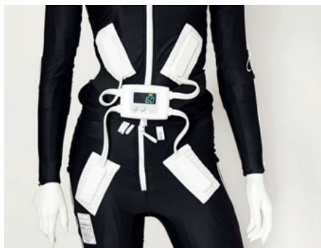
Fig. 1. The assistive technology comprising a tight-fitting, full-body garment and a control box worn at the waist. The garment has 58 stimulating electrodes integrated in relation to 40 different muscles, which enables TES therapy to be self-administered according to the individual profile programmed by a professional in a try-out session and stored in the control box (Mollii®, Inerventions AB, Stockholm).
