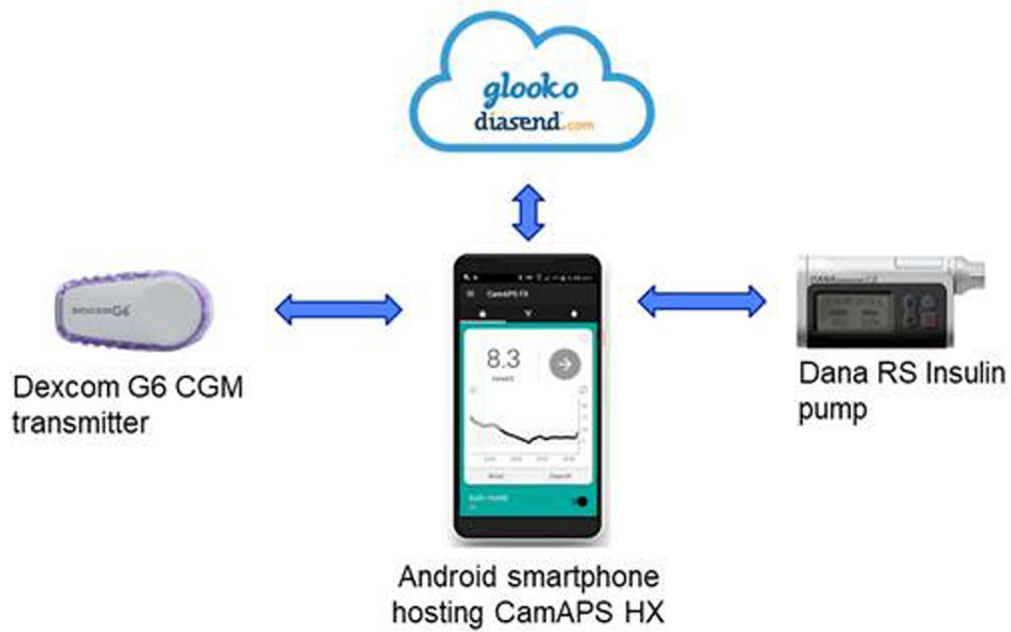
Extended Data Fig. 1 | CamAPS HX fully automated closed-loop insulin delivery system. CamAPS HX fully automated closed-loop insulin delivery system.
