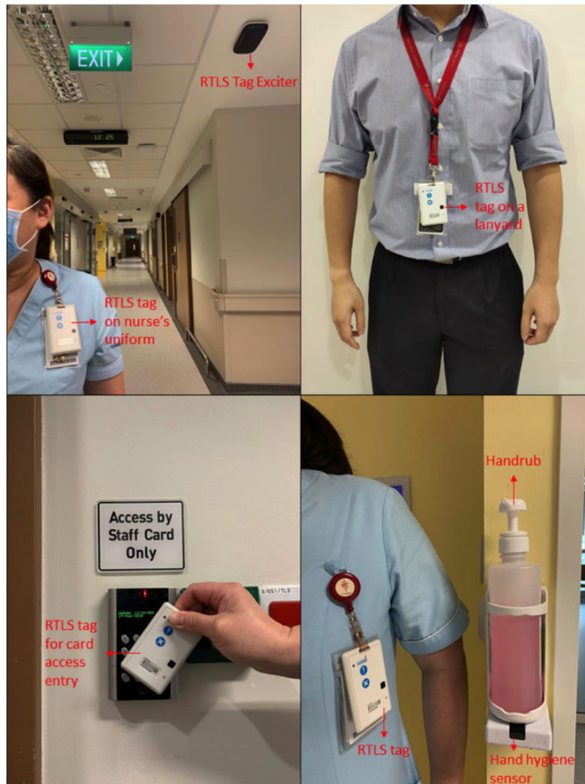
Figure 1. Photographs of the RTLS tag, the manner it is carried by staff, and its functions.
