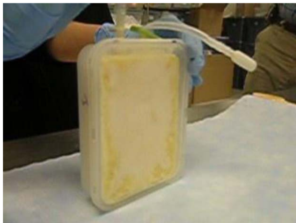
Fig. 1. Unique ruggedized lyophilization, storage, and administration container.
