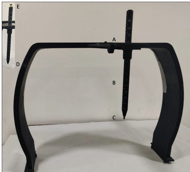
Figure 1: Respiframe (a). Horizontal bar (b). Pointer with scale to provide individualized tactile feedback to replicate DIBH position (c). Movable pencil in expiration (d). Movable pencil in DIBH position revealing (e). Fluorescent strip. DIBH: Deep inspiratory breath-hold
