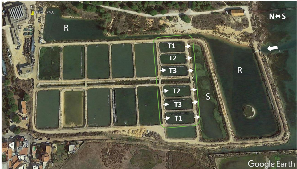
Fig. 2. Aerial view of the Aquaculture Research Station (Estação Piloto de Piscicultura de Olhão, EPP), south Portugal (37° 02'N; 07° 49'W) and location of earthen ponds with IMTA treatments (T1, T2, and T3). Arrows indicate water inlet and outlet; R - water reservoir; S – settling pond.
