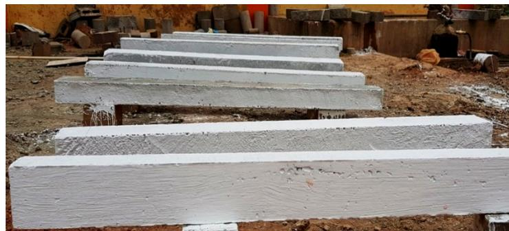
Figure 5. The RC beams cast for flexural testing.
