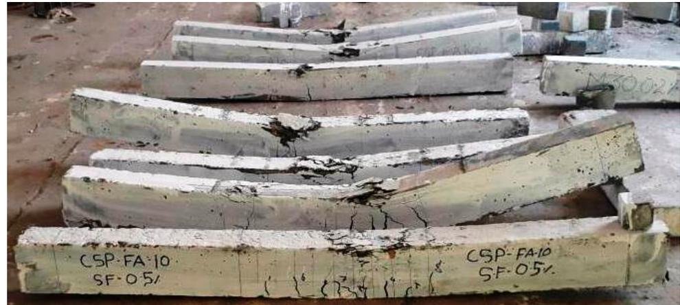
**Figure 7.** The beams tested for flexure (CS, CSF25, CSF 50, CSF 75, and CSF100).
