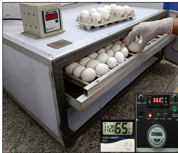
Figure 4. Storing a 0-day egg in a 37 \pm 1 °C egg incubator. This image shows an egg incubation setup. The inset images highlight the control panel and humidity meter. The control panel indicates temperature and humidity settings. The setup demonstrates the precision and care required while placing the eggs in the incubator to ensure successful hatching.
