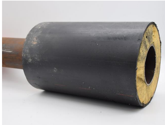
Figure 10. Photograph of the industrial insulated pipe sample.
