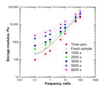
Figure 7. Isochronal storage modulus for ENR+SiO<sub>2</sub>, collected at different times during TRMS tests.
