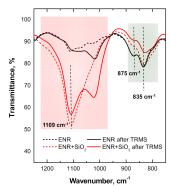
**Figure 9.** ATR-FTIR spectra for pristine (unfilled) ENR and ENR + SiO<sub>2</sub> composite before and after TRMS, in the range 1250–750 cm<sup>-1</sup>.
