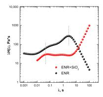
Figure 3. "Weighted" relaxation spectra for ENR and ENR + SiO<sub>2</sub> composite.
