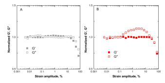
**Figure 4.** Large amplitude oscillatory shear (LAOS) rheological data for (**A**) pristine ENR and (**B**) ENR + SiO<sub>2</sub> composite.
