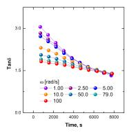
**Figure 10.** Multi-frequency plot for the variation of tan  $\delta$  as a function of time for ENR+SiO<sub>2</sub> system.
