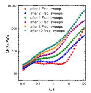
**Figure 5.** Weighted relaxation spectra for ENR+SiO<sub>2</sub> system subjected to subsequent frequency sweep measurements.
