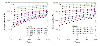
**Figure 6.** Time-resolved mechanical spectroscopy (TRMS) sweeps for ENR+SiO<sub>2</sub> at 180 °C: (**A**) storage modulus and (**B**) loss modulus.
