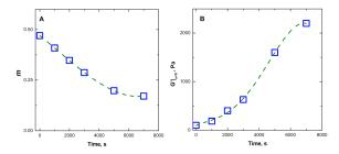
**Figure 8.** (**A**) Gradient (*m*) of the G' curves in the terminal region and (**B**) static modulus (G' |  $\omega$  = 0) for the for the ENR + SiO<sub>2</sub> melt.
