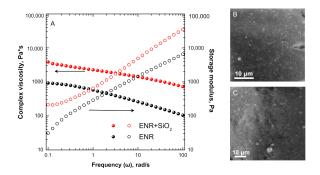
**Figure 2.** (**A**) Complex viscosity (full symbols) and storage modulus (empty symbols) and (**B**,**C**) SEM micrographs for ENR+SiO<sub>2</sub> composite at different magnifications.
