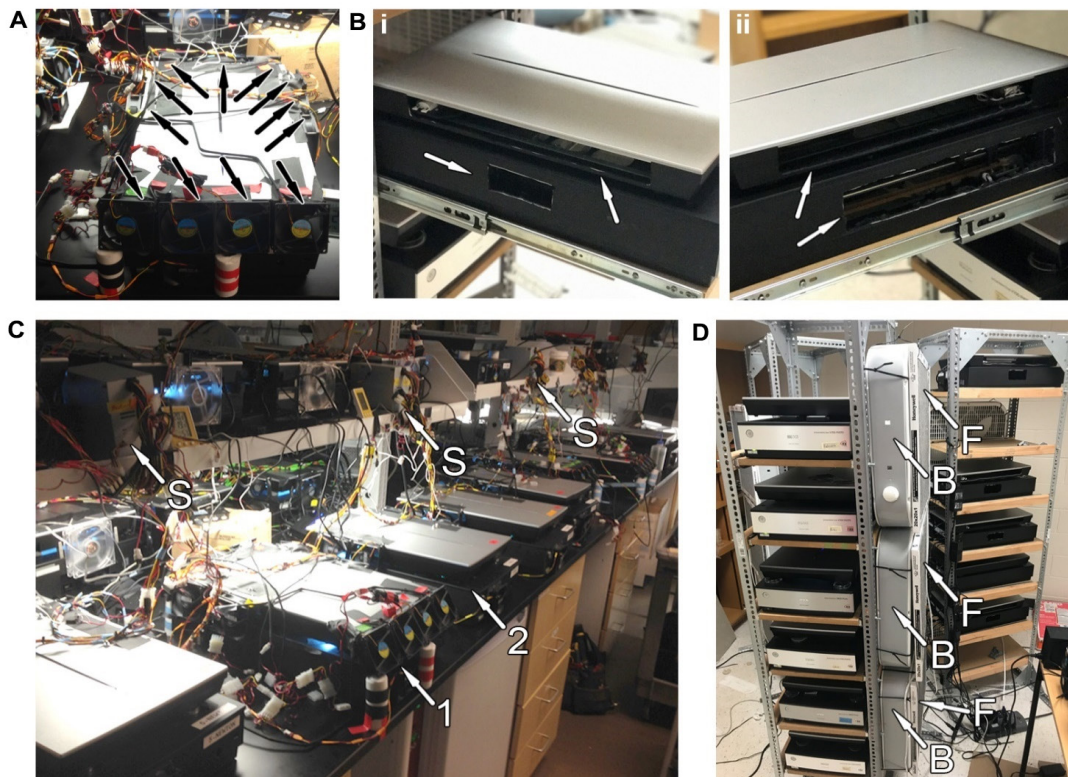
Figure 1. Lifespan machine designs. A. The original lifespan machine design, with pc fans connected to power supplies. B. The revised V700 lifespan machine design, with two cutouts (arrows) in the left side (i) and right side (ii). C. The V700 lifespan machine standard array. Computer power supplies (S) are wired to scanner fans. Some scanners (1) require additional fans to control temperature compared to others (2). D. New V700 lifespan machine array. Scanners are arranged on vertical racks with drawer slides for easy loading. Each box fan (B) covers two scanners and has an attached filter (F) to remove particulates from the airflow.
