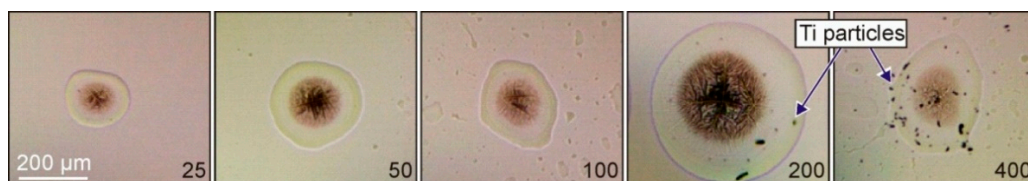
Figure 2. Optical micrographs of dried gel microdroplets on the acceptor slide produced with the same laser irradiation parameters ( \tau = 8 \text{ ns} , E = 20 \mu\text{J} , and F = 2.8 \text{ J/cm}^2 ) and different thicknesses of the Ti film on the donor slide. The numbers show the thickness of the Ti film in nanometers. In the last two images, Ti particles both inside and outside microdroplets can be seen.
