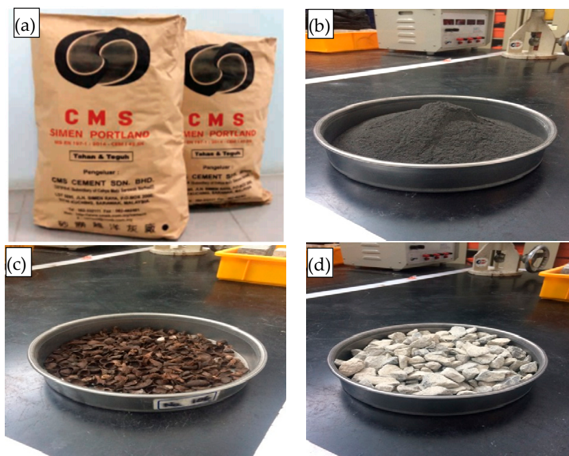
Figure 1. Materials used in the design mix, (a) OPC, (b) POFA, (c) OPS and (d) gravels.
