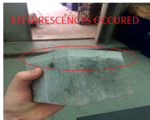
Figure 8. Calcium carbonate deposition layer on the specimen.
