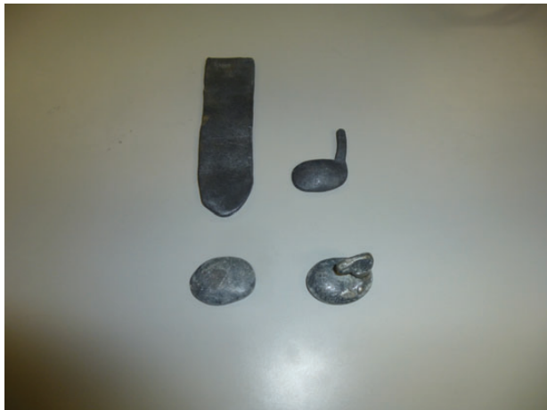
Fig. 1. Examples of lead blocks with various thicknesses and sizes to protect the lens.
