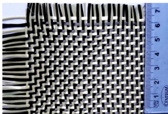
Figure 1. Photo of the SIGRATEX H W215-TW2/2 twill woven carbon-aramid fabric used to reinforce the laminated composite material tested (carbon fibres are black, aramid fibres are yellow).
