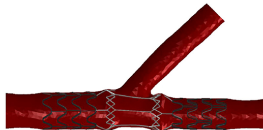
Fig 1. The creation of bifurcation model with side branch origin at 45 degrees, crimping of the stent and deployment of the stent in the bifurcation model.
