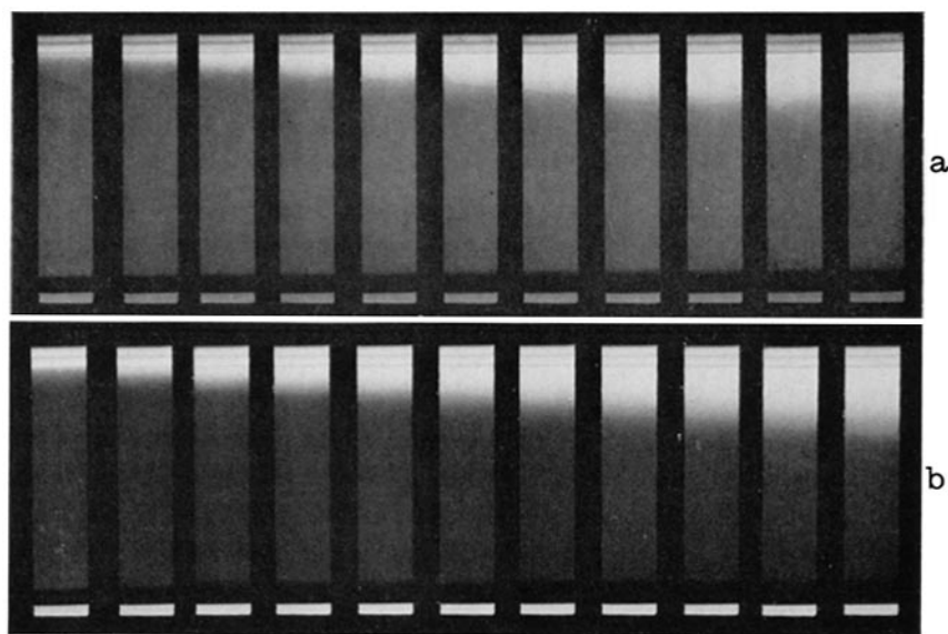
FIG. 2. Absorption photographs taken alternately at 5 minute intervals with a , red, and b , violet, light, showing sedimentation of the chlorophyll-protein in 0.25 per cent sodium dodecyl sulfate at pH 8.9. No differences are detectable in the two regions of the spectrum. The common sedimenting boundary was coincident with the protein boundary ( S_{20} = 2.6 \times 10^{-13} ) detected by the refractive index method, showing attachment of the pigment to the protein.
