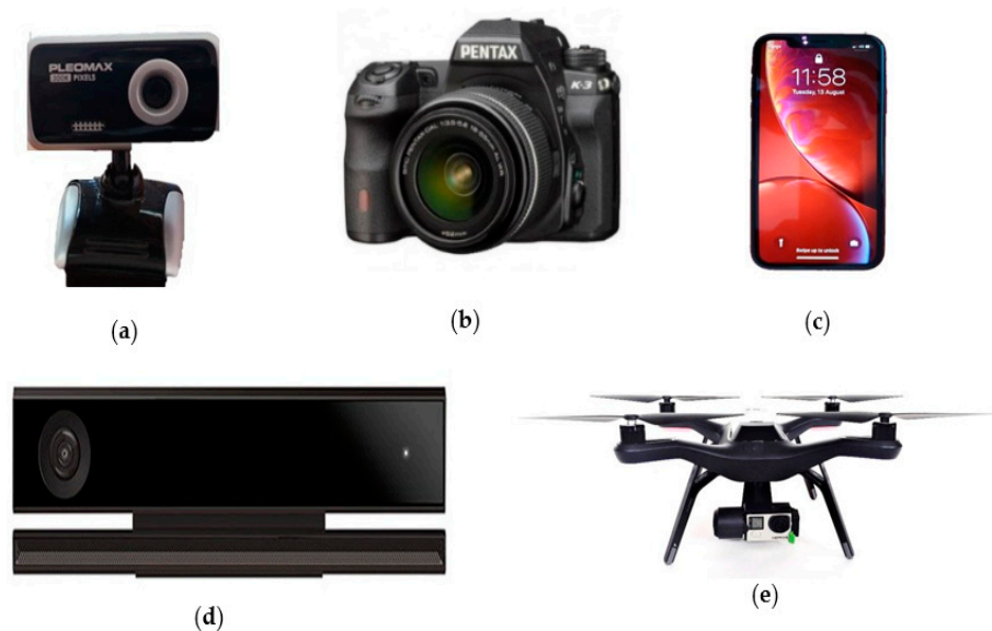
Figure 12. Different sensors used as a video camera. (a) Webcam, (b) digital camera, (c) smart phone, (d) Microsoft Kinect, and (e) UAV.
