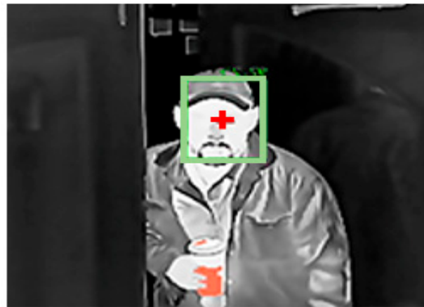
Figure 10. The thermal image presented in [98]. The face area is detected using a face detection algorithm and a point on the forehead (red color “+” mark) is selected for temperature measurement. Image courtesy of een.com.
