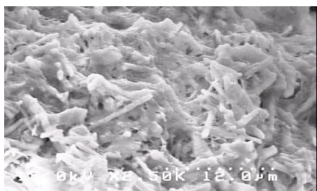
FIGURE 4: SEM micrograph of the matrix of copolymer with dispersed phase of hydroxyapatite needle-shaped particles.
