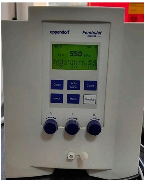
**Figure 3. FemtoJet microinjection system (Eppendorf) with the microinjection settings shown**
