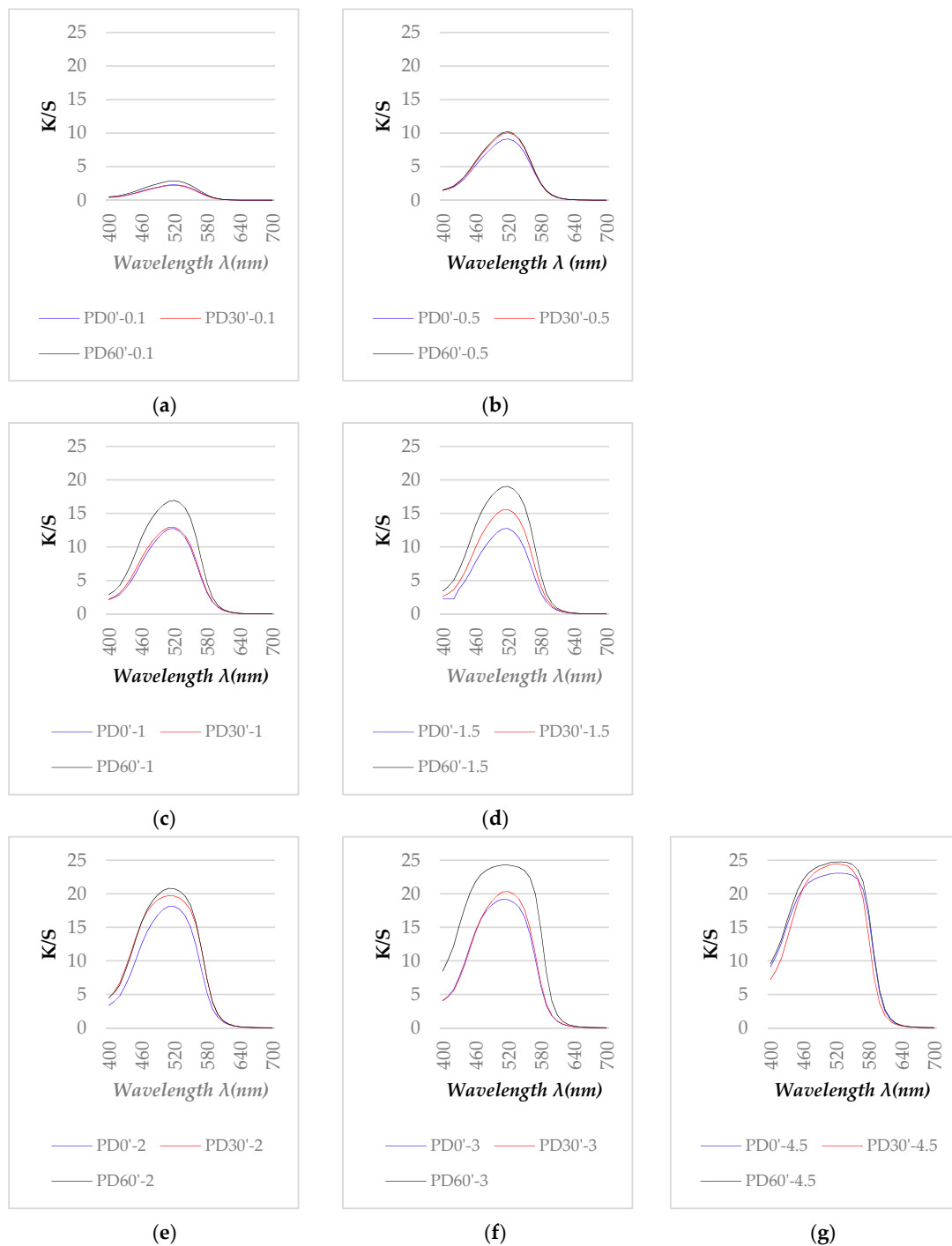
Figure 7. K/S spectra values of three sets of the dyed samples/rinsed in acetone (PD0', PD30', and PD60'): (a) samples dyed at 0.1% ( M = 0.1\% ), (b) M = 0.5\% , (c) M = 1\% , (d) M = 1.5\% , (e) M = 2\% , (f) M = 3\% , (g) M = 4.5\% . In all figures above, the blue curve is for the untreated polyester (PD0'), red for the plasma treated polyester for 30 s (PD30') and black for the plasma treated polyester for 60 s. (PD60').
