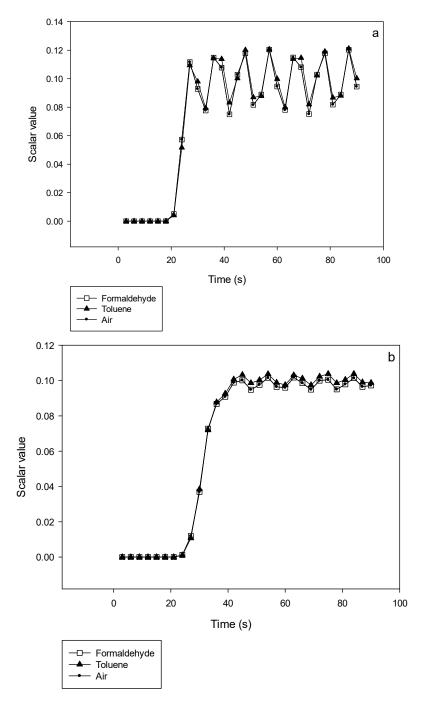
**Figure 8.** Comparison of the mixing's efficiency between formaldehyde, toluene and air being mixed with pure air at 25 NmL·min<sup>-1</sup>. Variations of the scalar value with time at the exit of a 2-stages (**a**) or 4-stages (**b**) device, illustrating that there is almost no time response difference between formaldehyde, toluene and air.
