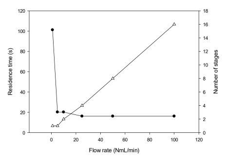
**Figure 7.** Number of stages ( $\Delta$ ) required for the oscillations of the scalar value at the micromixer's exit to be lower than 5% of the targeted value 0.1 at flow rates ranging from 1 to 100 NmL·min<sup>-1</sup>. Variations of the residence time (•) with the flow rate for the corresponding number of stages required. At 100 NmL·min<sup>-1</sup>, the 5% threshold is not reached: the percentage of oscillations is 6.1% after the 16th stage of mixing.
