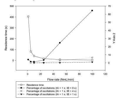
**Figure 6.** Residence time and percentage of oscillations around the targeted scalar 0.1 for flow rates ranging from 1 to 100 NmL·min<sup>-1</sup> at the exit of the 4th mixing stage. Percentage of oscillations is given for  $t_A = 1$  s and  $t_B = 9$  s, 4 s and 1 s.
