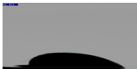
Figure 13. Contact angle confirming the wettability alteration to oil-wet after the aging process [34].
