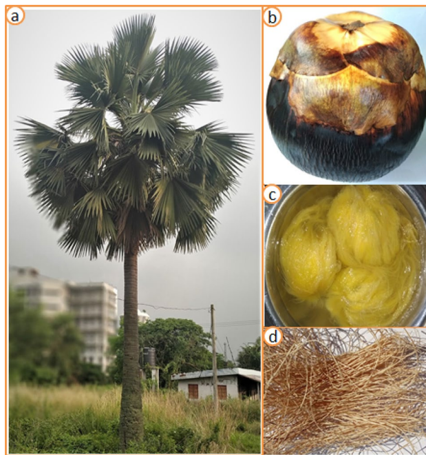
Figure 1. Corypha taliera fruit fiber extraction: (a) Corypha taliera plant; (b) Corypha taliera fruit; (c) Fruit seeds immersed into water; (d) Extracted dry fibers.
