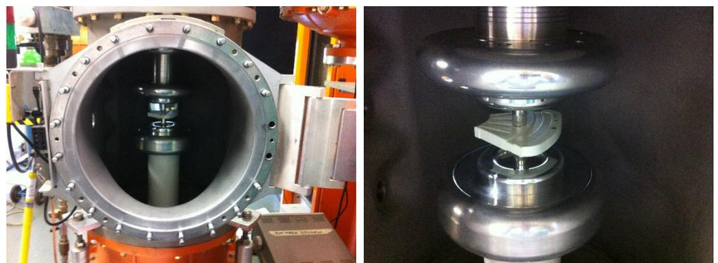
**Figure 2.** The barrier insulator disks during the electrical breakdown strength testing.
