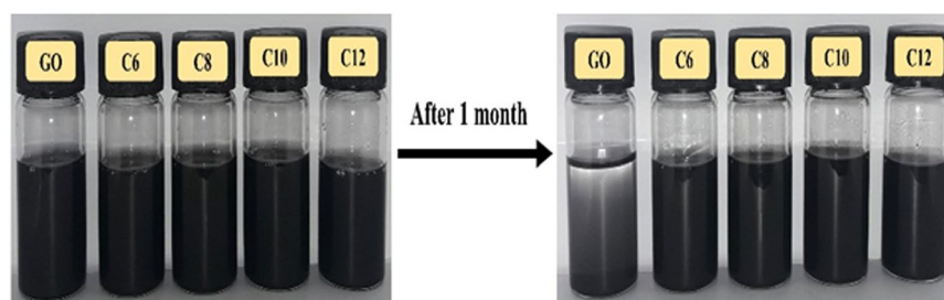
Figure 5. GO and rGO-T-C(n) dispersed in oil (left), after one month (right).
