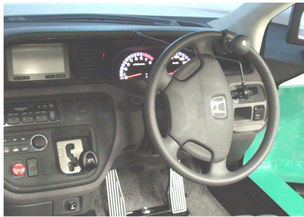
Figure 1 Modified driving simulator enabling patients with right or left hemiplegia to drive.
