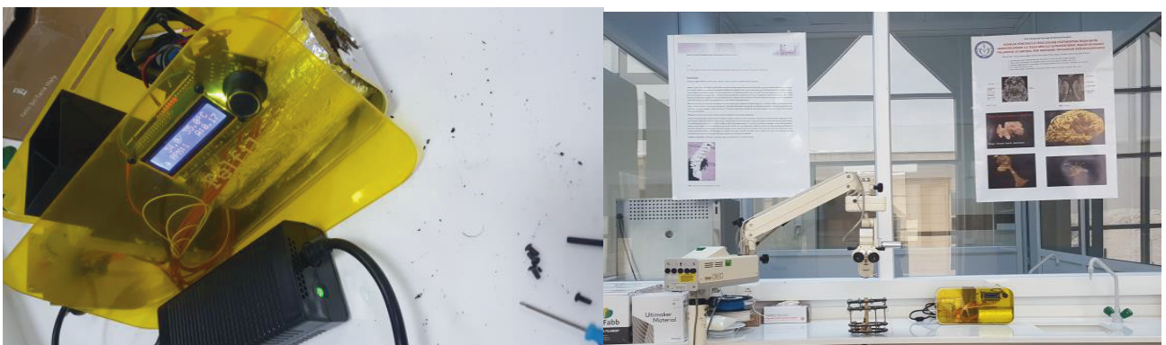
Figure 3. Extrusion device and HA-PLA filament preparation.
