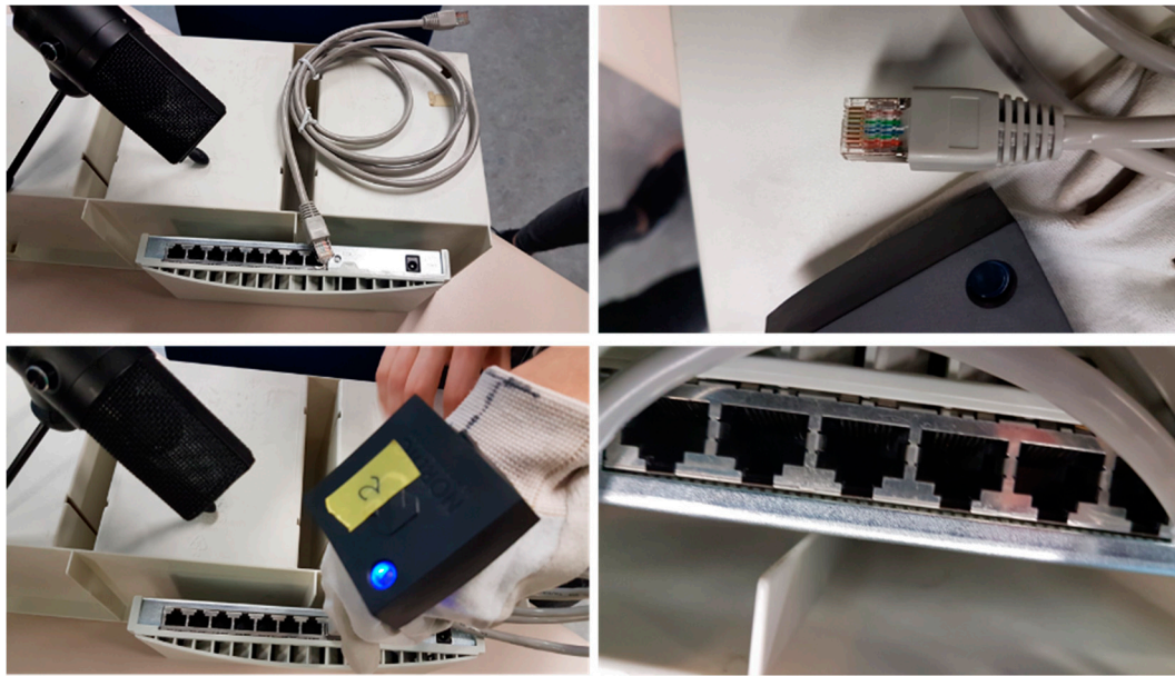
Figure 11. RJ-45 connection test bench: microphone, RJ-45 connector, sensory glove and network hub.
