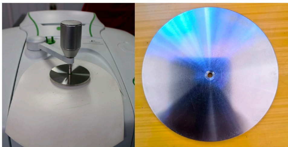
Figure 12. ZnSe ATR accessory (left) and the metal O-ring (right) in the study.
