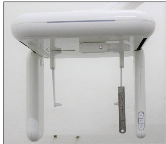
Figure 5: Head positioning device of Genoray CBCT Machine – Papaya 3D Plus utilized for uniform orientation of the head
