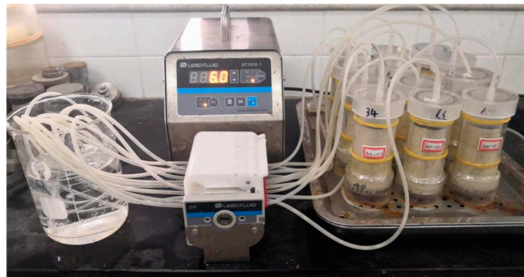
Figure 5. Grouting procedure of the peristaltic pump.
