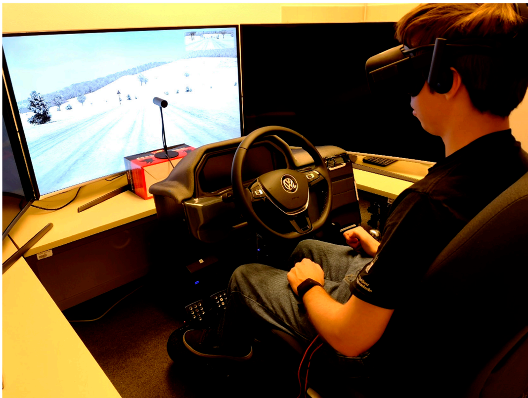
Figure 1. Participant prior to countryside ride in Nervtech™ driving simulator at the University of Ljubljana, Faculty of Electrical Engineering. The central UHD display was used to show the view of the driver from within the VR headset to the experimenter.
