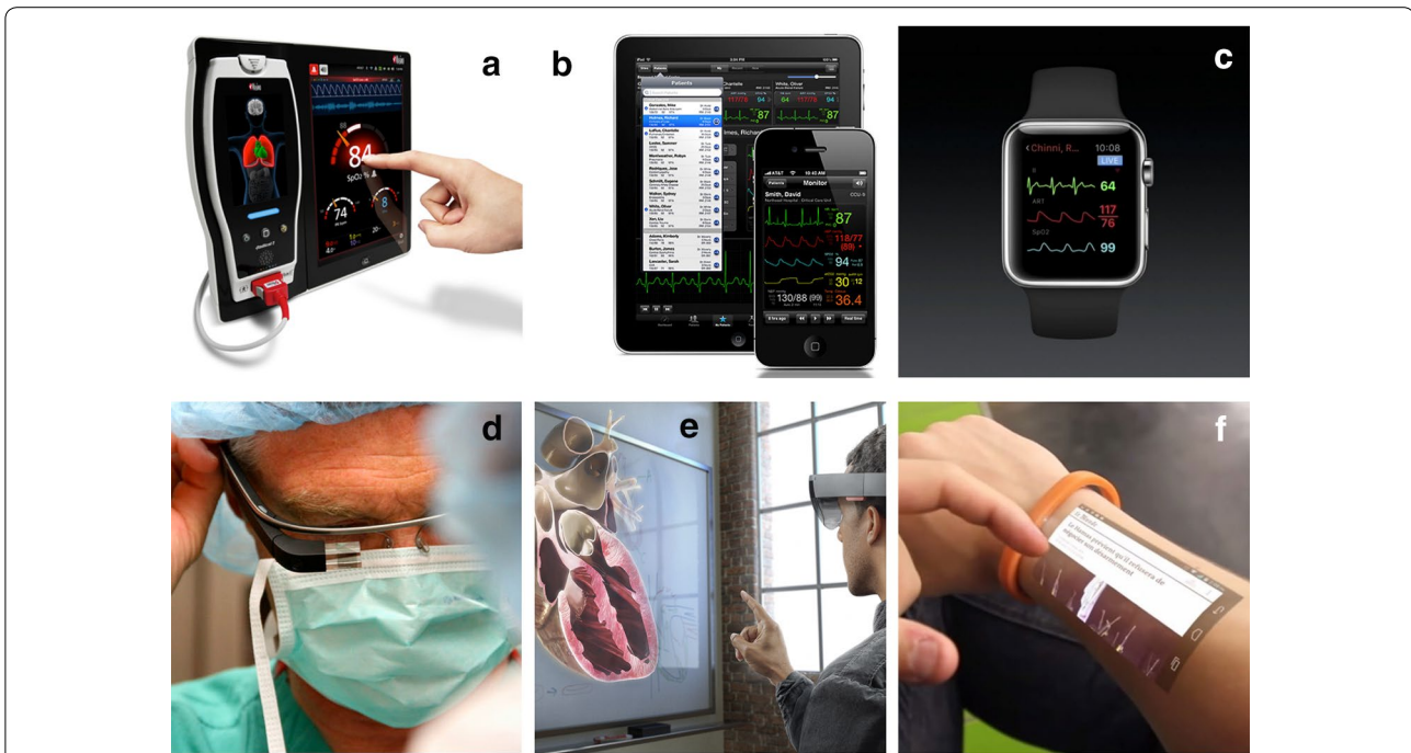
Fig. 4 Examples of digital methods to display monitoring information. a Bedside monitor, downloaded from Masimo.com; b tablet and cell phone, downloaded from Airstrip.com; c digital watch, downloaded from Apple.com; d connected glasses, downloaded from Google Images; e lenses allowing the visualization of images in three dimensions, downloaded from Microsoft.com; f laser pico-projection turning skin into a touch screen, downloaded from Cicret.com
