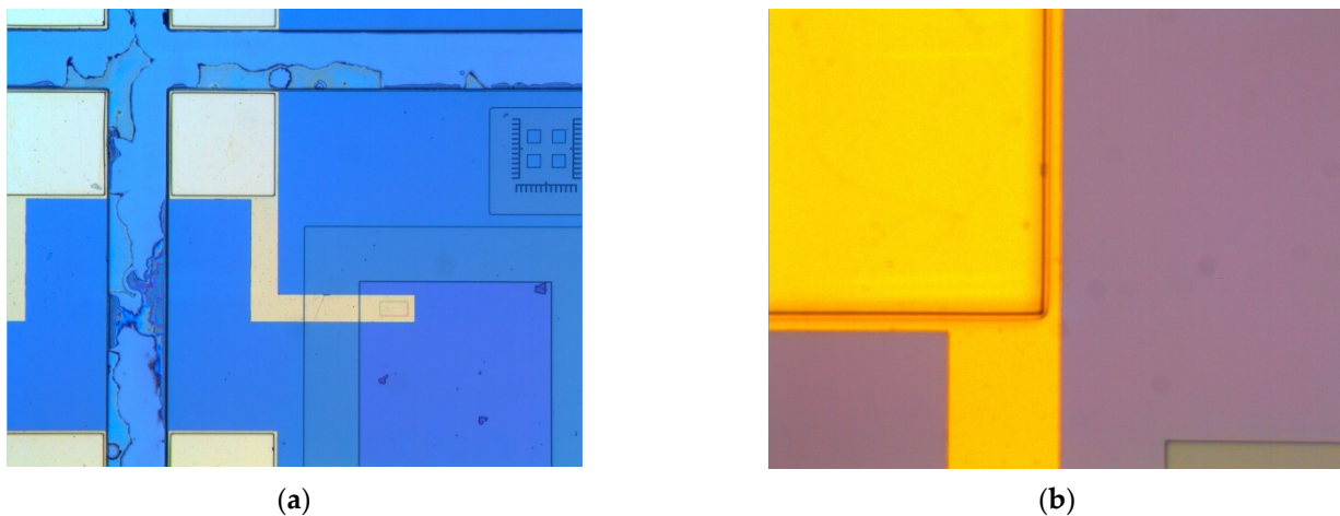
Figure 5. (a) Optical view of one external pad plus metallic trace to the source contact plus alignment sign and (b) details of the gold pad and gold trace to the source.
