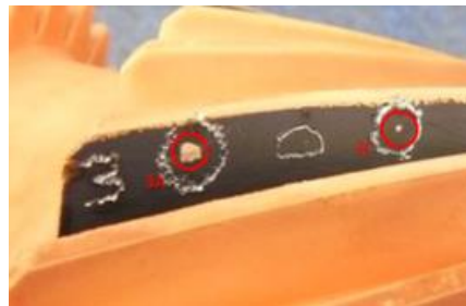
Figure 5. Gear sample with copper “spots” varying in size, representing chips locations close to pitch diameter of the gear teeth.
