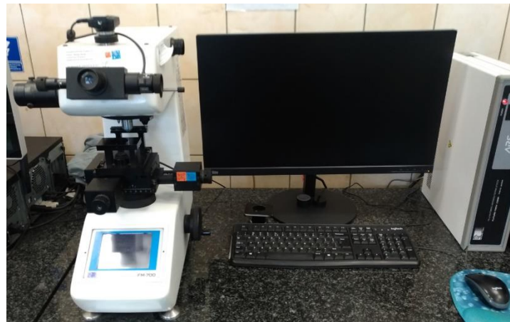
Figure 7. Hardness research station equipped with microhardness tester, Future-Tech Corp., Type: FM-700.
