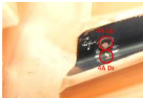
Figure 6. Gear sample with copper “spots” varying in size, representing chips in different locations on the gear teeth.
