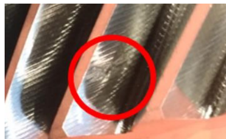
Figure 3. Bound chip on the tooth involute surface, after power skiving machining.
