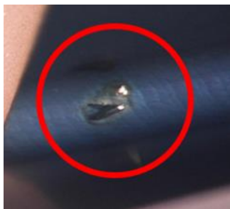
Figure 4. Bound chip on the tooth root, after power skiving machining.
