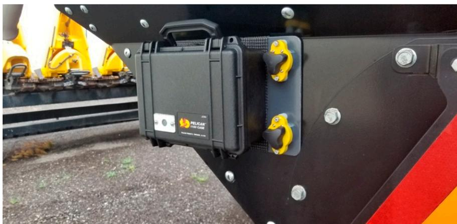
**Figure 1.** Data collection device mounted on the back of a piece of farm equipment.
