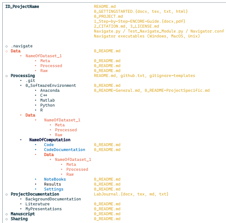
Fig. 6 | The standardized File System Structure (FSS) and associated pre-defined files. Standardized directory structure of the sFSS containing pre-defined files (gold), which include README files (in Markdown format) that provide a documentation template and instructions. Note that the pre-defined files in the 'Data' directories (orange) and the '0_SoftwareEnvironment' subdirectories are only shown once. The names of the directories 'NameOfDataset_1' and 'NameOfComputation_1' are placeholders and should be replaced with more descriptive
