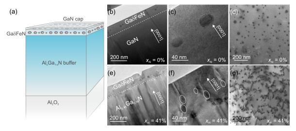
**Figure 1.** (a): Architecture of the investigated samples. Cross-section TEM micrographs of the samples grown (**b**,**c**): on GaN, and (**e**,**f**): on Al<sub>0.41</sub>Ga<sub>0.59</sub>N buffers, showing the embedded nanocrystals distributed in the Ga $\delta$ FeN layer. (**d**,**g**): Plan-view TEM images of the two samples, revealing an increased dislocation network for the layer grown on the Al<sub>0.41</sub>Ga<sub>0.59</sub>N buffer with respect to the layer grown on GaN.
