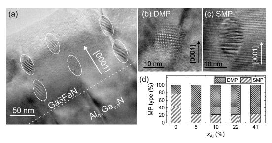
**Figure 5.** (a) Cross-section HRTEM image showing the distribution in pairs of prolate NCs along dislocations in the  $Ga\delta FeN/Al_{0.1}Ga_{0.9}N$  sample. (**b**,**c**) HRTEM images of nanocrystals with double and single Moiré-patterns, respectively. (**d**) Fraction of NCs displaying SMP and DMP as a function of  $x_{A1}$ .
