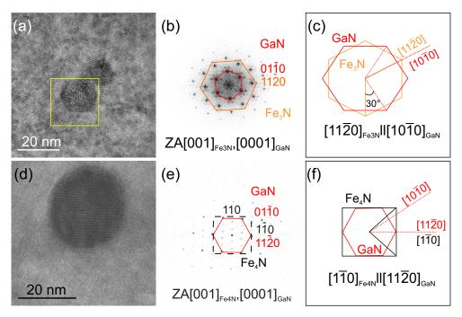
**Figure 6.** Plan-view HRTEM images of exemplary  $Fe_yN$  nanocrystals embedded in a  $Ga\delta FeN$  layer grown on (**a**) an  $Al_{0.1}Ga_{0.9}N$  buffer, and (**d**) GaN. (**b**,**e**) FFT of the images presented in (**a**,**d**), respectively, showing the epitaxial orientation of the NCs with respect to the GaN matrix. The FFT in (**c**) corresponds to the NCs marked by the square in (**a**). (**c**,**f**): Schematic representation of the epitaxial relation in (**b**,**e**).
