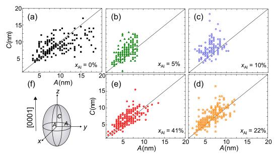
**Figure 4.** Size distribution of 200 NCs measured in cross-section HRTEM for  $x_{Al}$  in the buffers equal to: (a) 0%, (b) 5%, (c) 10%, (d) 22%, and (e) 41%. The dimensions A and C correspond to the schematic representation depicted in (f) and correspond to half the size perpendicular and parallel to the [0001] growth direction, respectively.
