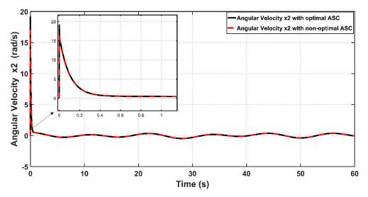
Figure 13. Behavior of joint velocities for optimal and non-optimal ASC.
