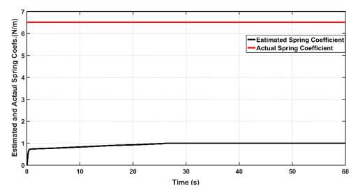
Figure 17. Actual and Estimated Spring Coefficient for Bicep muscle of PAM actuated robot based on ASC.
