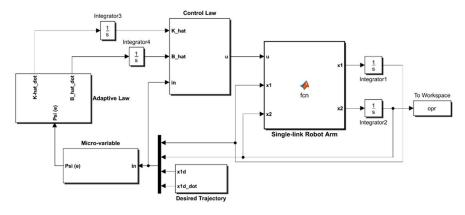
Figure 3. Simulink Model of Adaptive Synergetic Controlled Robotic System.
