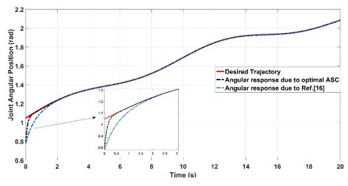
Figure 18. The tracking response based on optimal ASC and the compared controller of reference [16].
