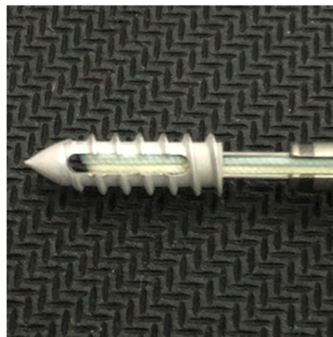
Fig. 1. The processing drawing and picture of HP Mg suture anchor.
