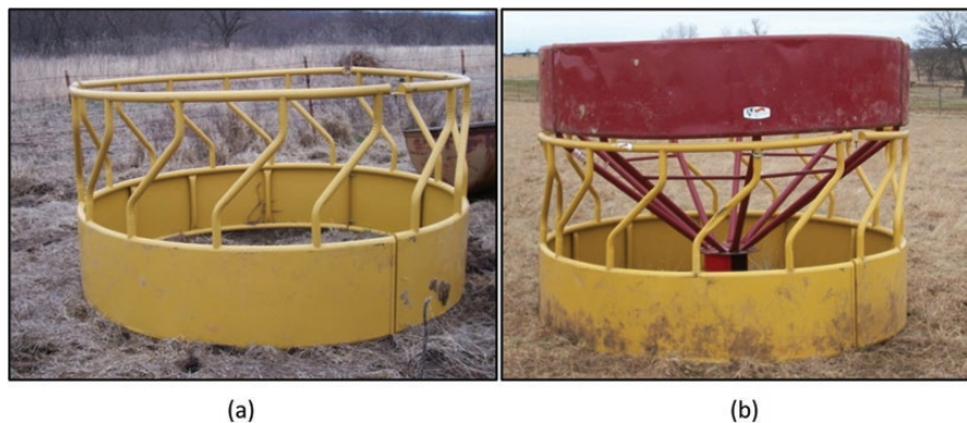
Figure 2. Round bale feeder designs used in experiment 2: (a) sheeted bottom steel ring feeder; RING (Franklin Industries, Montecello, IA); (b) sheeted bottom steel ring feeder equipped with a cone insert; CONE (Franklin Industries, Montecello, IA).
