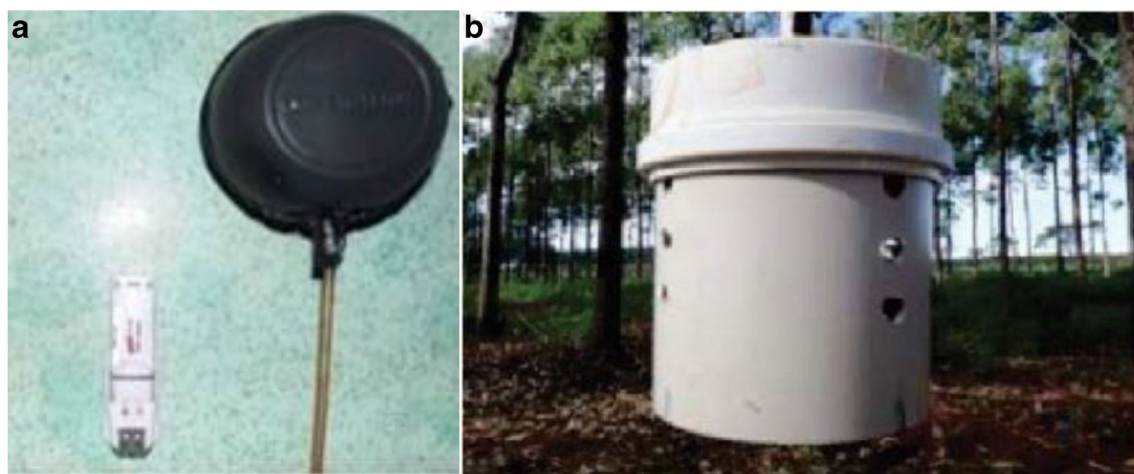
Fig. 2 Component devices of the micrometeorological station. a Digital thermo-hygrometers with data logger, black globe. b Perforated micrometeorological shelter next to the data logger
