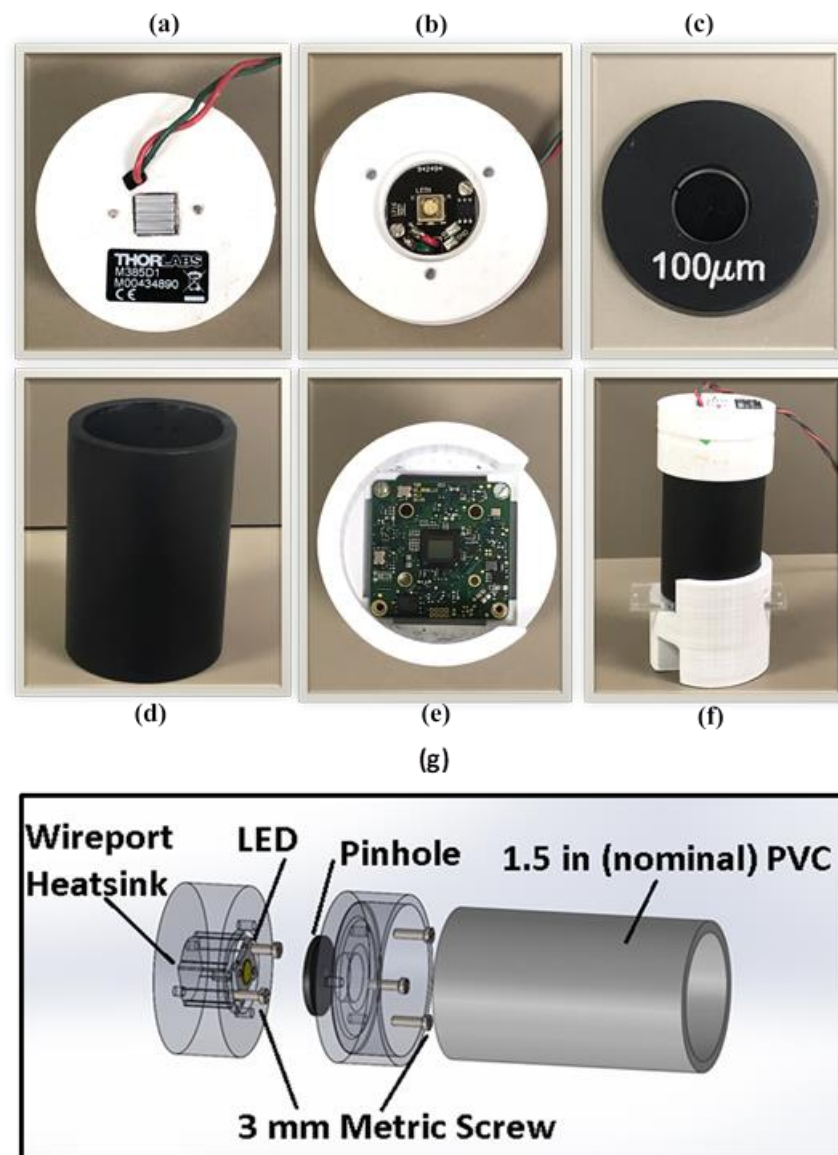
Figure 1. Components utilized in the development of portable imaging setup. (a) The 3D printed component containing the heat sink (b) LED fitted inside the custom-built housing. (c) 100 microns sized pinhole (d) PVC pipe (e) CMOS sensor mounted on a 3D printed base part (f) The complete lensless imaging setup with an antibody-coated microfluidic chip. (g) 3D sketch of the mechanical design of developed lensless imaging setup.
