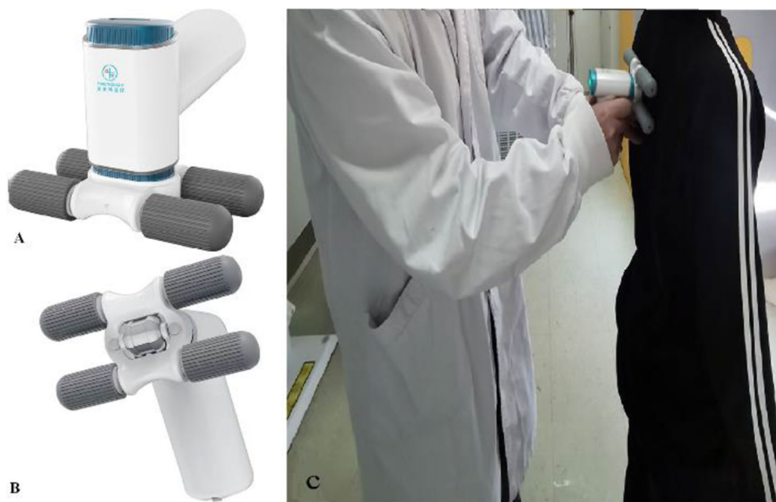
Fig. 2 Illustration and operation of 3D-SSS. (A) Housing, switch and LED indicator of the device; (B) One light-sensitive roller and four balance rollers of the device; (C) Operator moves the device along the patient's spine from T1 to L5
